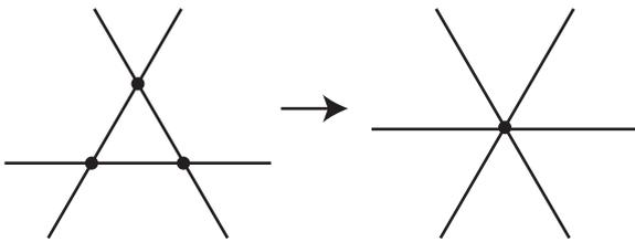
Figure 3. The number of line segments and points decreases by 3 and 2 respectively if a line intersects an existing point.
